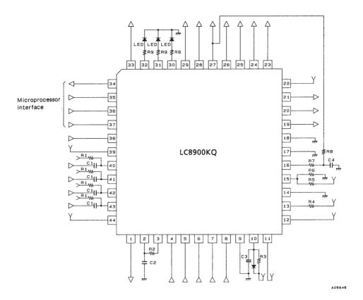
$\ast$  Apply the power to AV\_{DD} and two DV\_{DD}s simultaneously, or a latch up will occur.  $\ast$  The allowable current to BSA, CD, and BSB pins is 8 mA.
