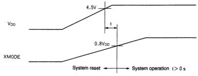
Each input pin will be accessible after XMODE turns to be on to start the system.
