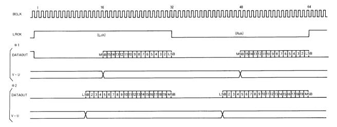
\*1: This operation timing is based on the following conditions: OUTMODE pin level=low and DI1 bit=low \*2: This operation timing is based on the following conditions: OUTMODE pin level=high and DI1 bit=high V = Validity flag output. U=User's bit output.
